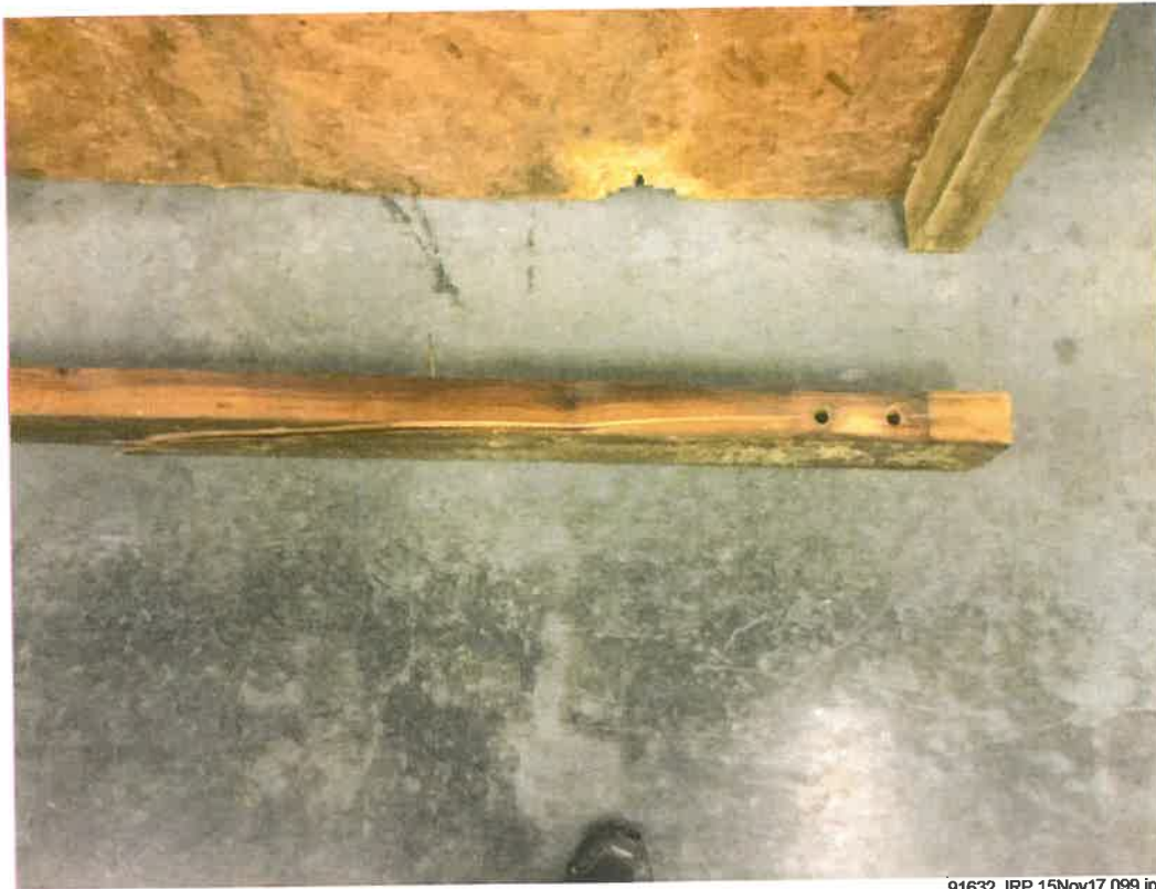
Figure 1. Crack in 3 rd web member from east wall of fifth truss from the north end.
